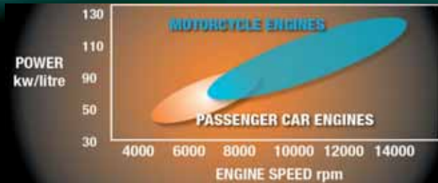
Motorcycle engines run faster and have a higher power/size ratio than car engines
